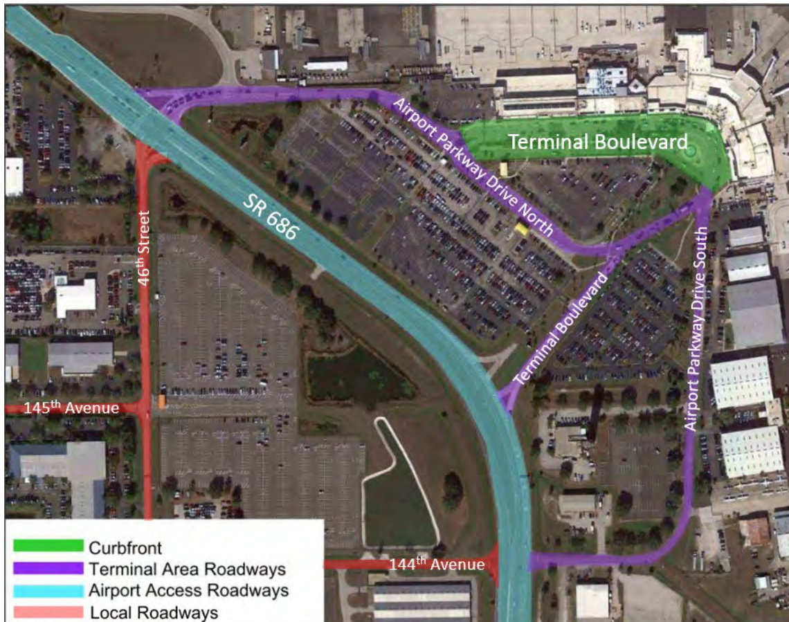
Figure 2.3-3: Terminal Access Roadways
